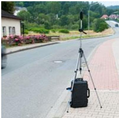
The outdoor noise kit consists of a sound level meter with all its standard accessories and additionally a waterproof PELI carrying case with rollers that has external connections for a microphone and for the power supply. Therefore, it is possible to leave the meter itself in the case to protect it from the weather. In the case, there is a waterproof charger and two additional rechargeable 12 V lead batteries to supply the meter with power for up to 10 days.
